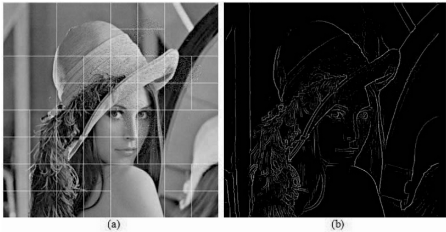
Fig. 12.9. (a) Segmentation of image Lena into sharp, blurred and noisy (homogeneous regions). (b) Edge detection results based on the homogeneous regions after the segmentation.
