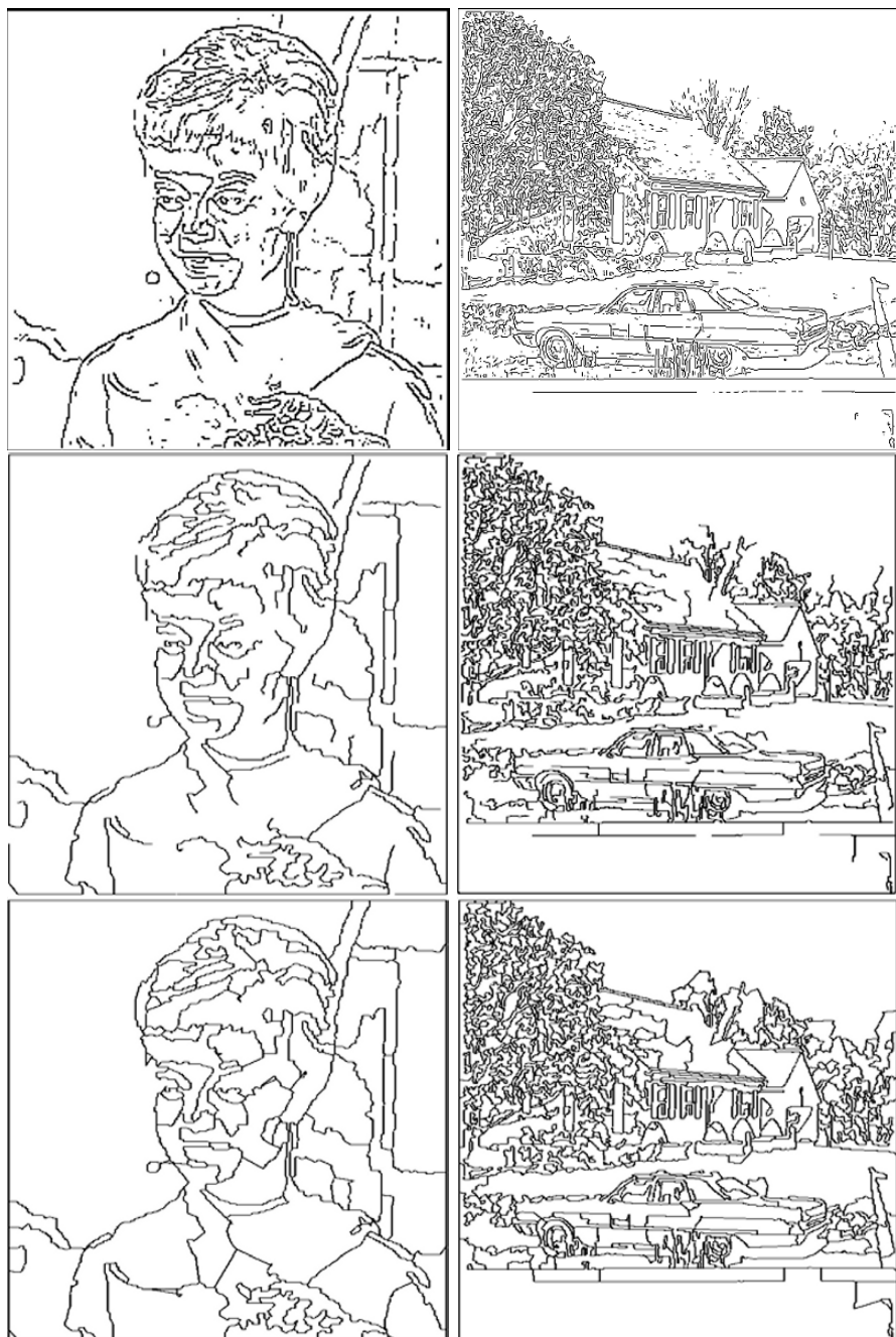
Fig. 11.5. (top) Input edge points (6387 and 34827 points). (middle) Filtered MST (4964 and 26689 edges). (bottom) Final closed contour representation (5052 and 27257 edges).
