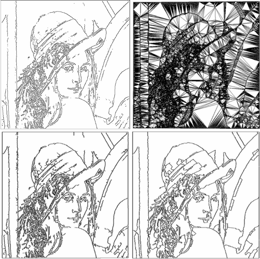
Fig. 11.4. ( top – left ) Input edge points, 21393 points. ( top – right ) Triangular mesh. ( bottom – left ) Minimum spanning tree, 21392 edges. ( bottom – right ) Final closed contour representation (after filtering the MST and closing open boundaries), 18517 edges.
