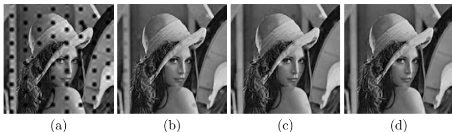
Fig. 21.3. (a) Lena -image after loss of packet 5. (b) Damaged Lena -image repaired with the bilinear interpolation [3] (PSNR = 30.88 dB). (c) Damaged Lena -image repaired with our previous interpolation method based on the globally dominant correlation direction [6] (PSNR = 31.59 dB). (d) Damaged Lena -image repaired with our proposed reconstruction method (PSNR = 31.97 dB)
