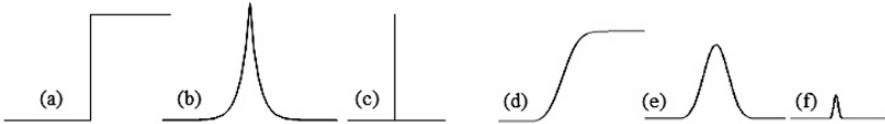
Fig. 12.1. (a) step edge, (b) crest-line edge and (c) impulse edge. (d) Blurred step edge (ramp edge), (e) blurred crest-line edge and (f) blurred impulse edge.
