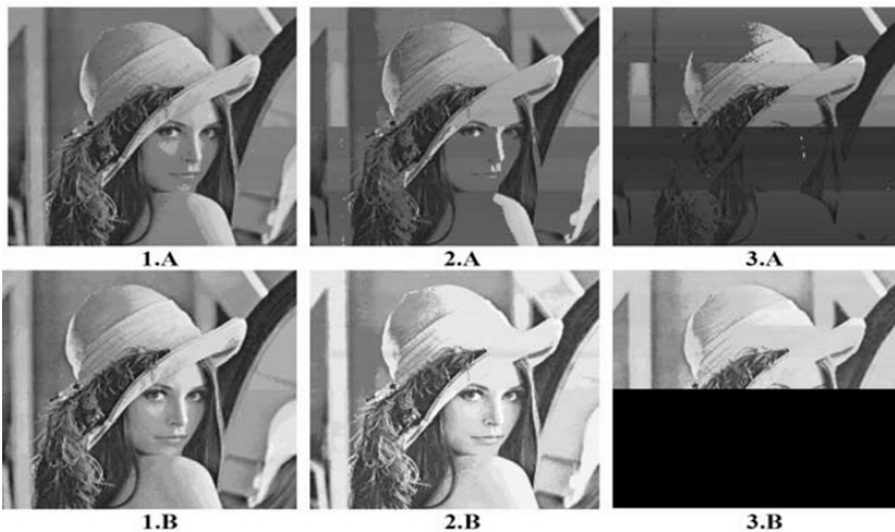
Fig. 27.6. PFM and PWM encoding as a function of the intensity-to-time conversion factor \tau . The left image represents the highest value of \tau with preceding images representing a lower value.
