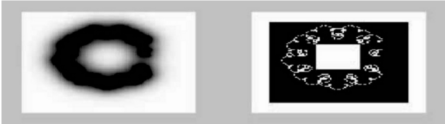
Fig. 16.4. Scale aspect: Hull effect (with inner and outer markers). Left: final state. Right: Shape and marker. Parameter c = 8 .
